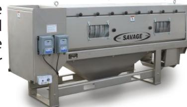
The Savage Inspection Table (model 520S) allows for visual inspection of the shelled nuts as they transit the vibrating table. Operators can quickly remove unwanted shells and nuts into conveniently located chutes on one or both sides of the table. The table with hopper measures 59" high x 108" long x 37" deep.
