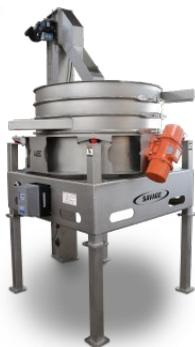
The Savage Meat Sizer (model 150S) is our smaller-scale meat sizer. It does a great deal of work in a very small footprint (47" high x 63" long x 21" deep). This machine conveys shelled nut-meats across a series of four vibrating screens of increasing size. Screens can be customized to your needs. An optional large-capacity receiving hopper can be integrated.
