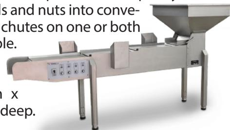
The Savage 522S Packaging/Inspection Table is often the final station of a nut processing plant. A single operator is able to visually inspect shelled nuts, and weigh them as they fall into a box or bag. The operator can also control the rate of flow from the large hopper. This station measures 65" high x 38" wide x 40" deep and is shown with the 704S 8-foot Bucket Elevator.
