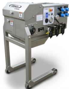
Savage Crackers come in two sizes, both of which will put old-fashioned mechanical crackers to shame. The 252S (shown) will crack pecans at 750 nuts per minute, while the 238C (opposite page) cracks nuts at 400 per minute.
