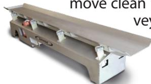
The Savage Meat Sizer (model 148S) is the newest addition to the Silverline family. It is built for industrial-speed sizing. The stacked sizing screens can be swapped out quickly. You can sort two, three, four or more sizes and the discharge chutes can be oriented in almost any direction. Shown with 704S Elevator.
